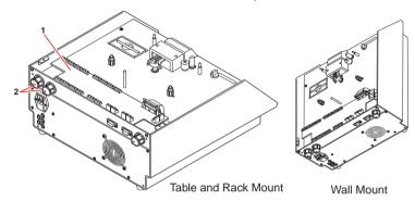
Figure 3-10: Relay Panel (Cover Removed)
