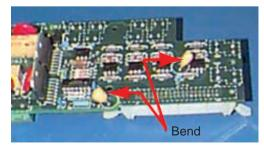
Figure G-7. Bend Capacitors on I/O PCB
