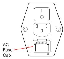
Figure 9-9: AC Fuse Cap
