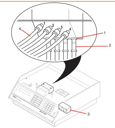
Figure 9-11: Microtube Assemblies
