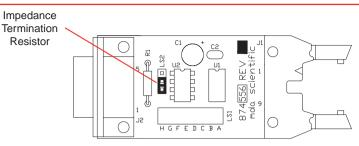
Figure E-6: CM4 RS-485 Interface Board Impedance Resistor Location.
