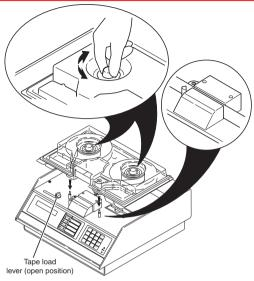
Figure 9-4: Installing the Carrier
