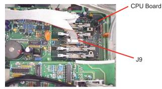
Figure G-8. LonWorks Ribbon Cable Connected to CPU
