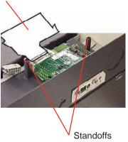
Figure G-4. Insulator Installation
