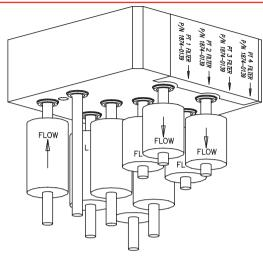
Figure 9-8: CM4-P Filter Block
